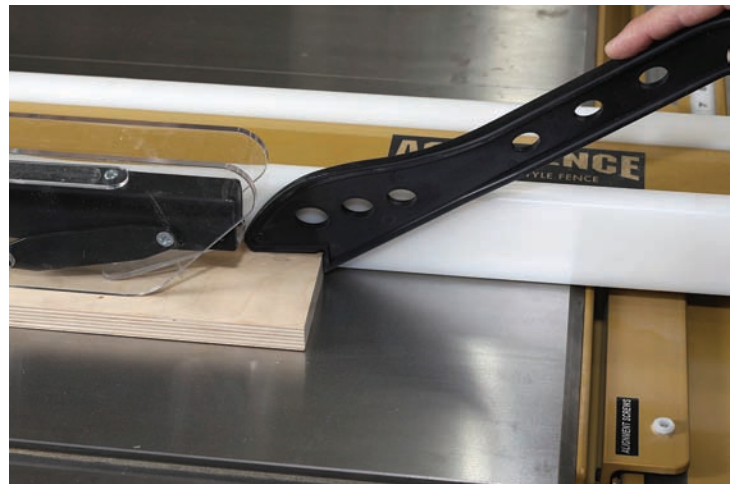
16 Use a push stick to distance your hands from the blade when ripping narrow stock.
