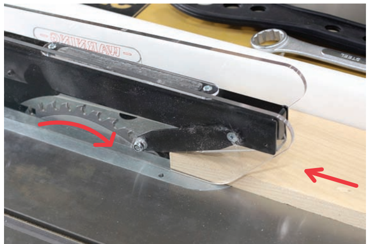
6 Always feed the stock against the direction of the power tool rotation.
