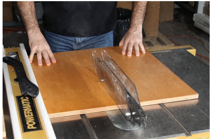
18 Make certain the workpiece is supported before starting the saw.
