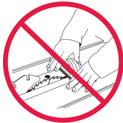
4 Never cut stock freehand. Always use the fence or miter gauge to support the workpiece.
